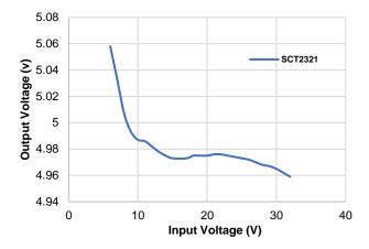
Figure 8. Line Regulation (IOUT=2A)
