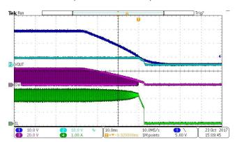
Figure 15. Power Down VIN=24V, VOUT=5V, IOUT=2A
