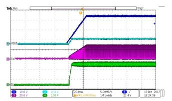
Figure 14. Power Up VIN=24V, VOUT=5V, IOUT=2A
