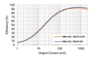
Figure 1. SCT2321 Efficiency, Vin=12V
