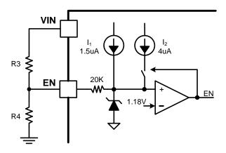
Figure 9. Adjustable VIN UVLO
