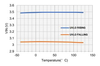
Figure 6. VIN UVLO vs Temperature
