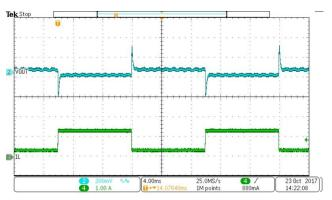
Figure 13. Load Transient VOUT=5V, IOUT=0.5A to 1.5A, SR=250mA/us
