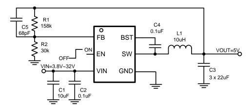
Figure 11. 24V Input, 5V/2A Output
