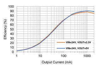
Figure 2. SCT2321 Efficiency, Vin=24V
