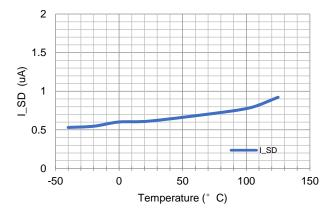
Figure 3. Shut-down Current vs Temperature
