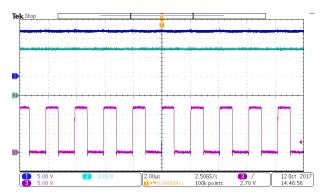
Figure 10. SCT2321 Switching Node Waveform
