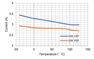
Figure 5. Peak Current Limit vs Temperature
