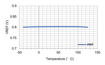
Figure 4. Reference Voltage vs Temperature
