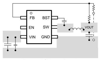
Figure 18. PCB Layout Example
