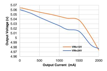
Figure 7. Load Regulation, (VOUT=5V)
